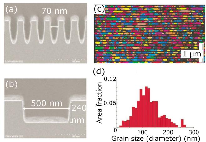
FIG. 1. (Color online) Cross-sectional SEM images of damascene trenches with linewidths of (a) 70 nm and (b) 500 nm. (c) A grain map of the 70 nm Cu wires obtained by electron backscatter diffraction. Each color represents a different crystal orientation. (d) A histogram of the grain size distribution derived from the image in (c).
