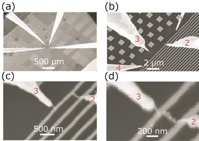
FIG. 2. (Color online) (a) SEM image of the Cu wires being contacted by the four probes. (b) An enlargement of the image in (a). In the four-terminal  $I$ - $V$  measurements, the current flows between tips 1 and 4, and the voltage drop is measured between tips 2 and 3. [(c) and (d)] Images of the voltage probes 2 and 3 approaching each other. The probe spacings are (c) 750 nm and (d) 70 nm.
